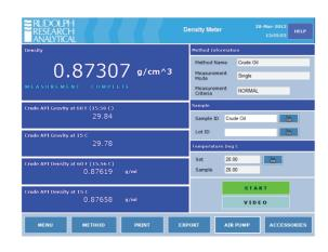
The historical method for the measurement of API Gravity has been the hydrometer. However, the low precision of the hydrometer as the prices of crude oils increase make this method obsolete. Additionally, the large sample volume required, the large quantities of solvents needed for the cleaning of the hydrometer column, and the need for a dozen or more different hydrometers to cover the entire API range has made using this method completely impractical in today's petroleum laboratories.
